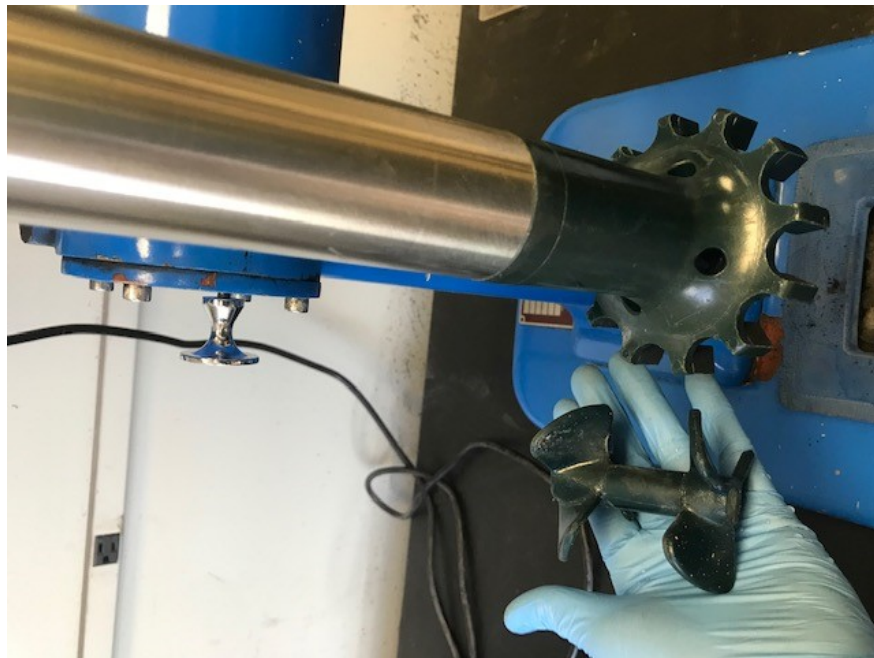
Figure 4: Impeller used for attrition scrubbing
